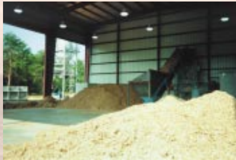
Wood chips are brought to the power plant by the truckload on a regular basis. When up and running at full capacity, the plant can consume 200 tons of recycled wood per day.
