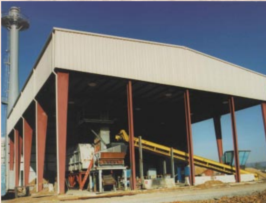
Wood chips are sorted by size and fed to the walking floor machine to begin the process of generating power with recycled wood.
