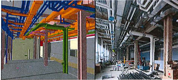
Figure 4 – 3D Collision Coordination using BIM
