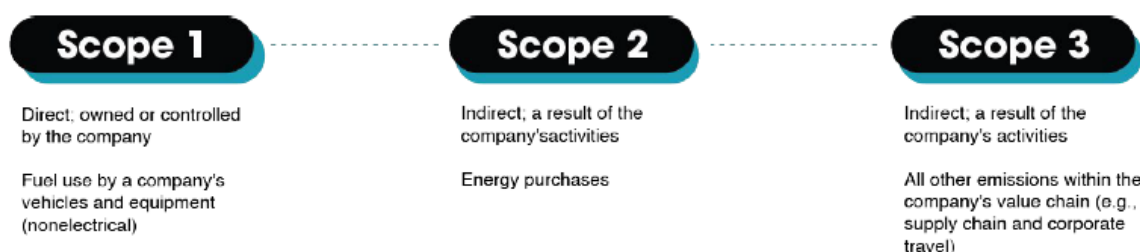
Fig. 2 – Direct and Indirect greenhouse gas emissions as defined in the GHG Protocol
